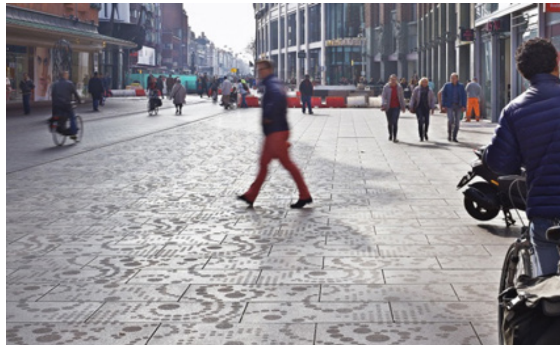
Reference for pavement pattern for the Brewhouse plaza - using bushhammered finish of the pattern in the flamed granite paving. Hop plant pattern to be used
